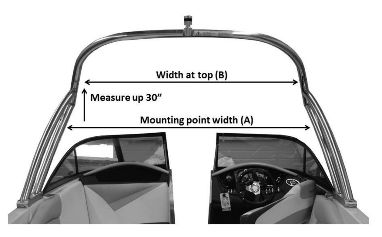
Note: Height for Bimini top when folded from mounting point A: 45"
